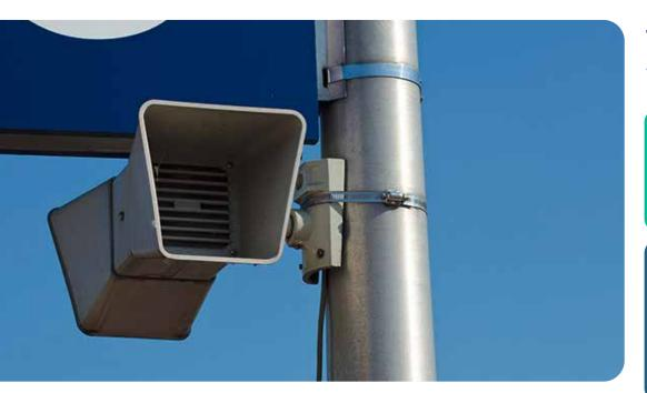
DAKS-AudioConnect connects the telephony world with an existing PA infrastructure or loudspeaker system. Thus, prepared messages or live announcements can be output directly from the telephone to PA loudspeaker systems. In the process, these are optimally synchronized acoustically.
